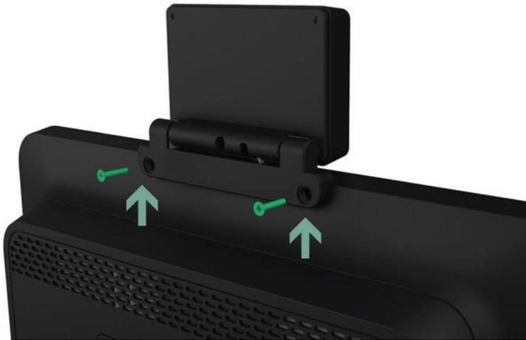
Step 5: Attach the screws in the accessory bag to protect the mera and adjust the angle as needed.
