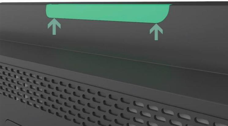
Step 2: Remove the selected peripheral interface cover from the side of the main device.
